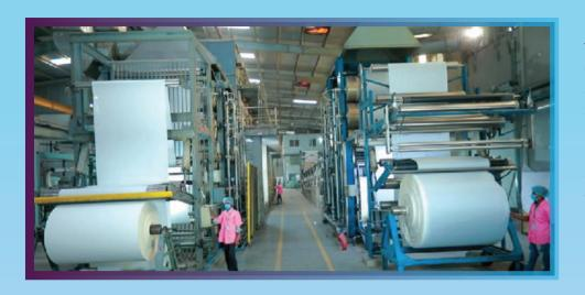
Back Process of fabrics is done for making the fabrics ready for dye and print through the state-of-the-art machines such as Singeing and Desizing from Osthoff, Germany, Continuous Scouring and Bleaching as well as Mercerizing from Benninger of Switzerland.
